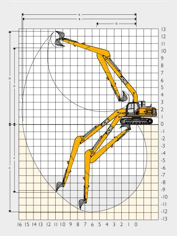
Working dimensions calculated using 980/B0092 GP bucket on Monoboom and T.A.B. and 980/A0391 GP bucket on LR.
