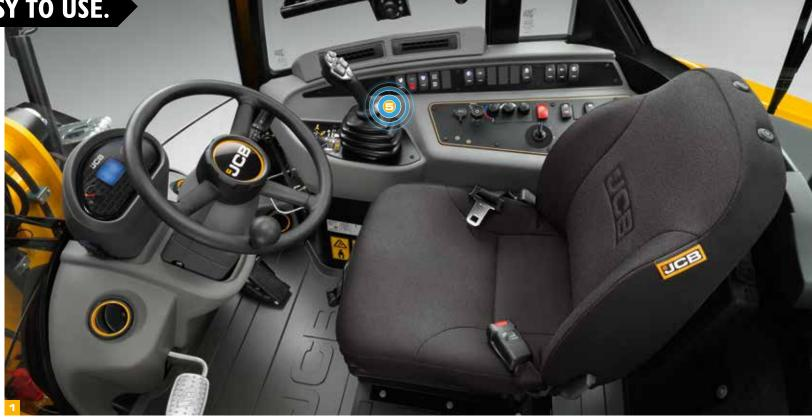
A stylish modern central dash display combines analogue dials and a colour LCD screen which can display machine health details, service requirements, operating information and more.
