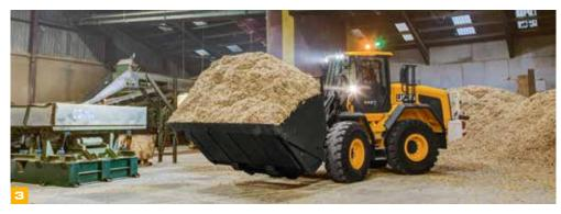
A Specify your perfect loader arm: Z-bar linkage (ZX) for high breakout applications or high torque (HT) for parallel lifting and multi-attachment work.
