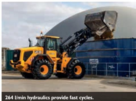
264 l/min hydraulics provide fast cycles.
