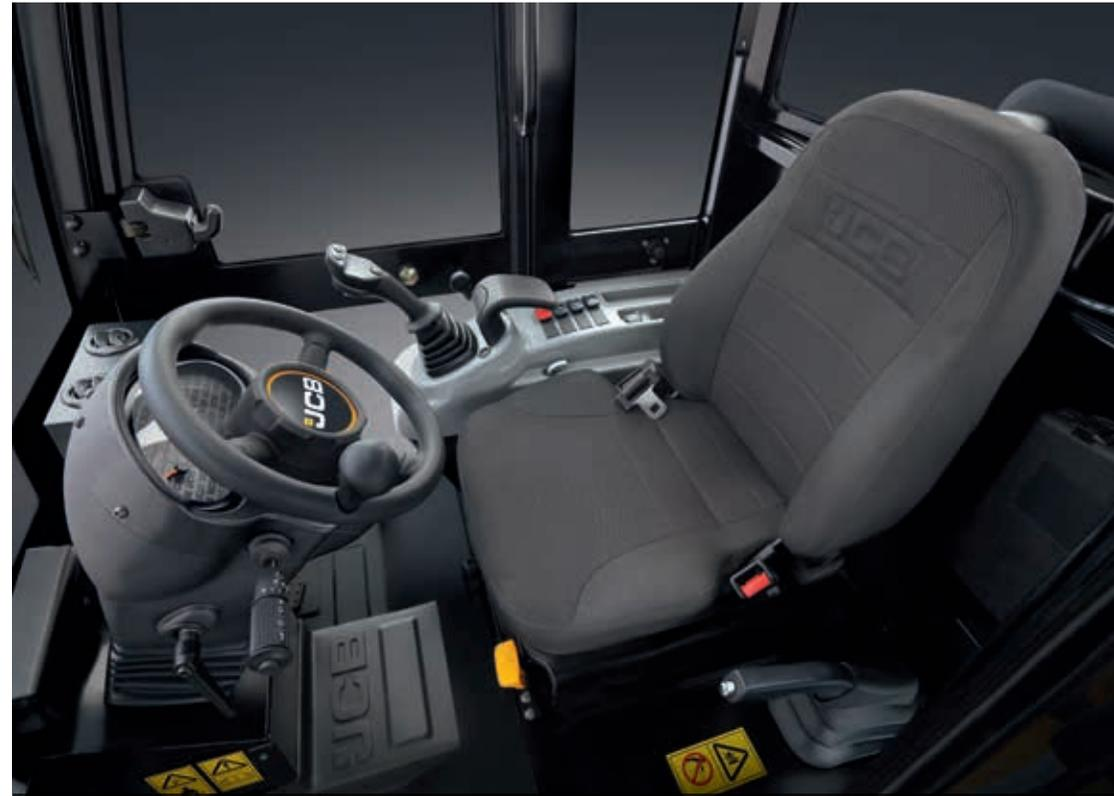
The new JCB 403 benefits from a comfortable and spacious cab. Our tilting steering column is easy to adjust for an ergonomic driving position.
