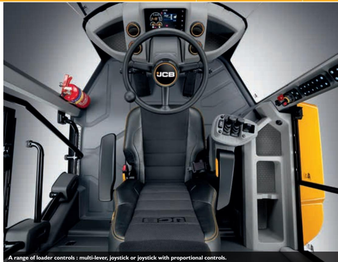
A range of loader controls : multi-lever, joystick or joystick with proportional controls.
