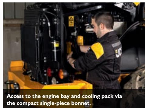
Access to the engine bay and cooling pack via the compact single-piece bonnet.
