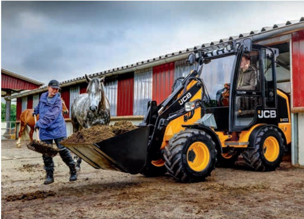
Compact wheel base and 45 degree steering articulation help to ensure tight turning circles and superb manoeuvrability.
