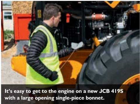
It's easy to get to the engine on a new JCB 419S with a large opening single-piece bonnet.
