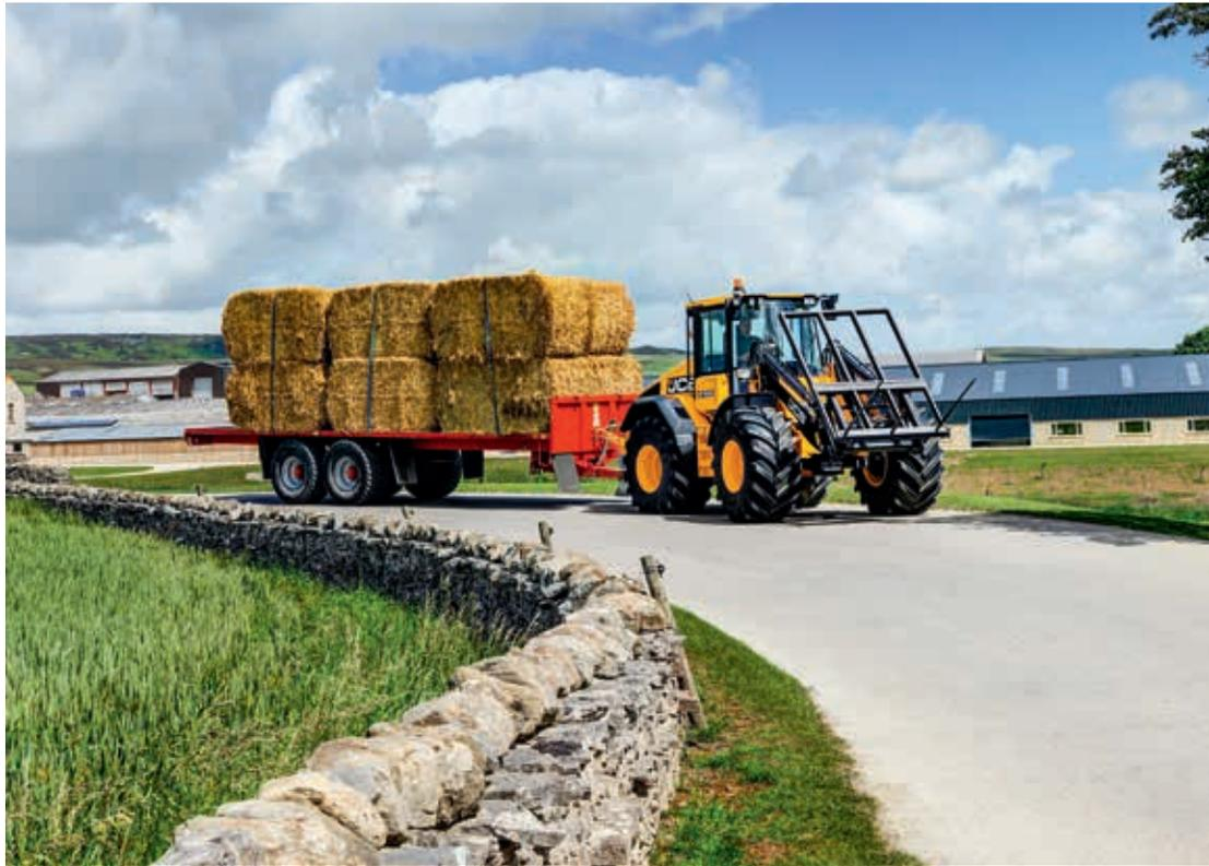
Optional 10 tonne hydraulic or mechanical tow hitch with hydraulic trailer brakes and 12V trailer electrics further improve versatility.
