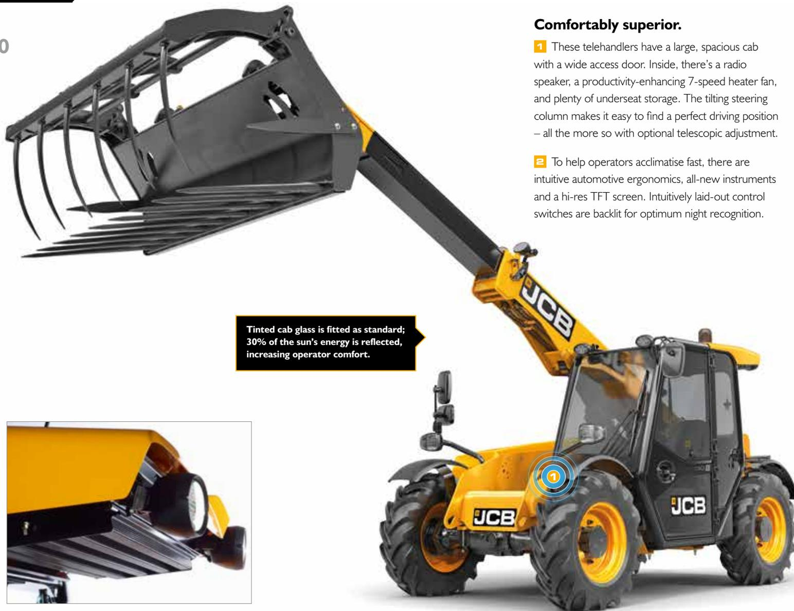
Tinted cab glass is fitted as standard; 30% of the sun's energy is reflected, increasing operator comfort.
