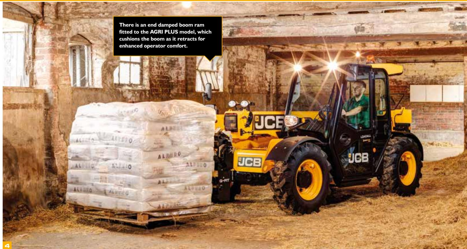
There is an end damped boom ram fitted to the AGRI PLUS model, which cushions the boom as it retracts for enhanced operator comfort.
