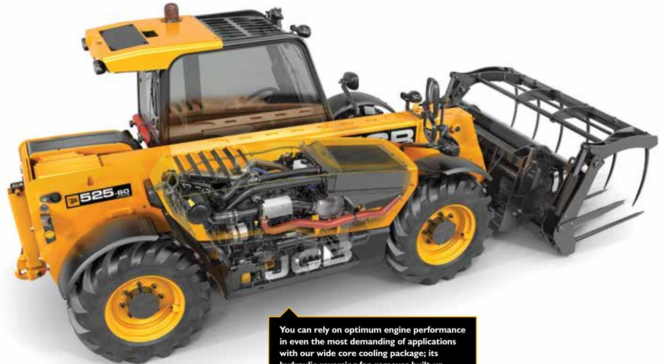
You can rely on optimum engine performance in even the most demanding of applications with our wide core cooling package; its hydraulic reversing fan removes built-up debris from the cooling pack efficiently.
