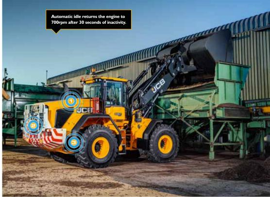
A new auto engine shutdown feature saves fuel by switching off the engine when the machine is left idling. Idle time can be set by the operator from the cab seat.
