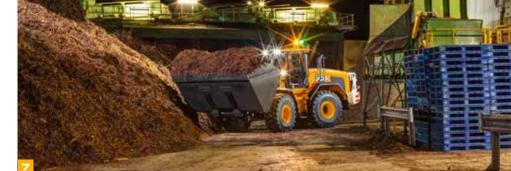
Specify your perfect loader arm: Z-bar linkage (ZX) for high breakout applications or high torque (HT) for parallel lifting and multi-attachment work. High lift or Super high lift option equips your 457 for applications involving high loading heights, such as hopper and lorry loading.
