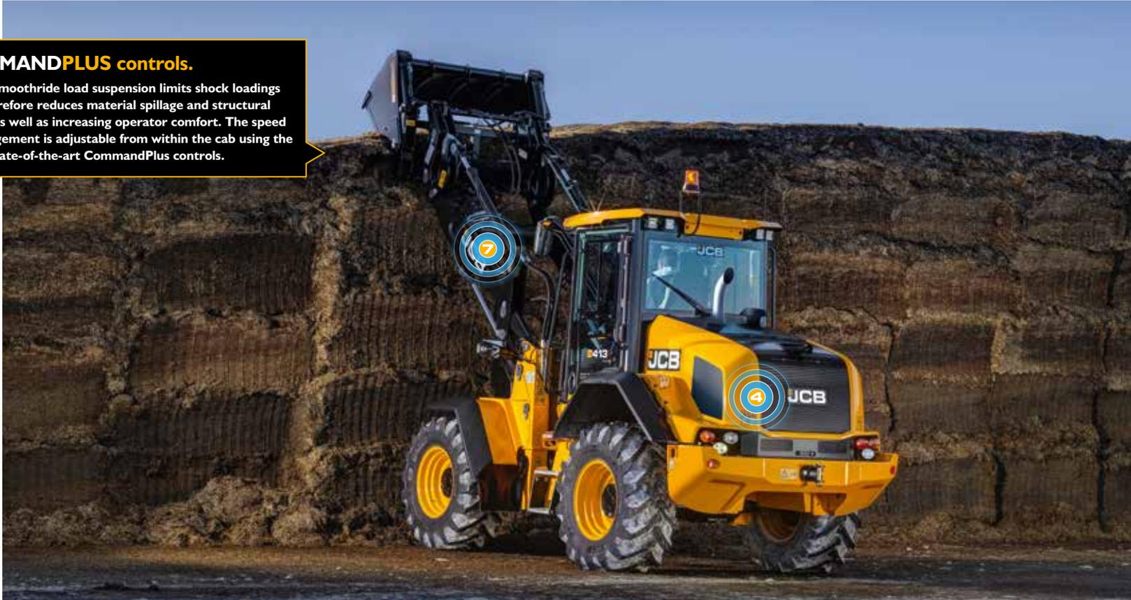
**4** A new auto engine shutdown feature saves fuel by switching off the engine when the machine is left idling. Idle time can be set by the operator from the cab seat.
