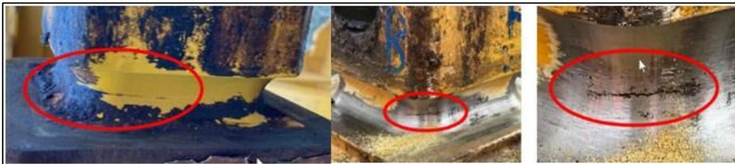
To put it out of service, either cut the groove or the top of the fishplate with an angle grinder or a torch. **A photo of the destruction of the fishplate will be required with the completion form.**
