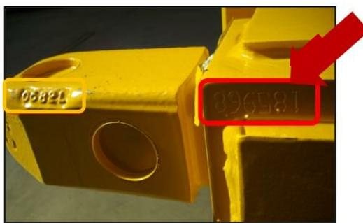
In order to facilitate the follow-up of inspections of a fleet of chassis masts and to serialize them, Potain will send you serialization plates (see photo below), which we ask you to install on each S41A and S41A1 chassis mast in your fleet. The plate should be installed as shown below and a photo of the plate will be requested in the proof of completion.
