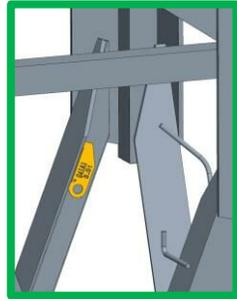
Code for the unequipped basic chassis mast: 84045630
